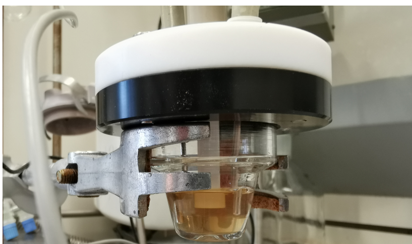
Fig. 3.1: Inert gas cell designed for electrochemical analytics and use in electrocatalytical experiments
